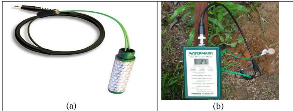
**Figure 2.** (a) Watermark<sup>TM</sup> soil tension sensor and (b) Watermark<sup>TM</sup> equipment for reading soil water potential ( $\Psi_m$ ).
